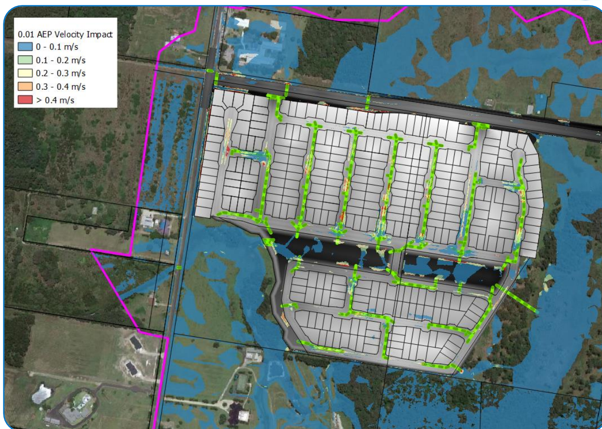
Figure 6.13 1% AEP Velocity Afflux Plot
