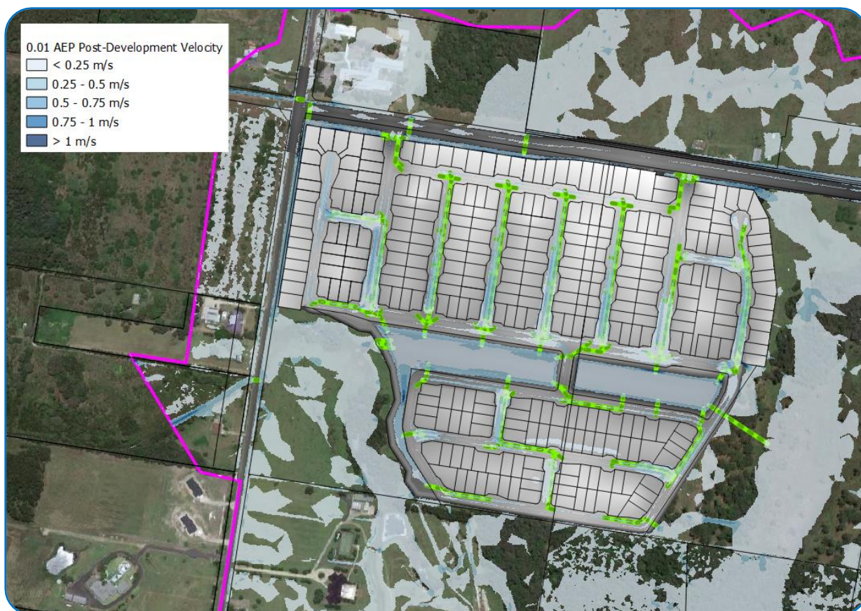
Figure 6.11 0.01 AEP Post-Development Peak Flood Velocity
