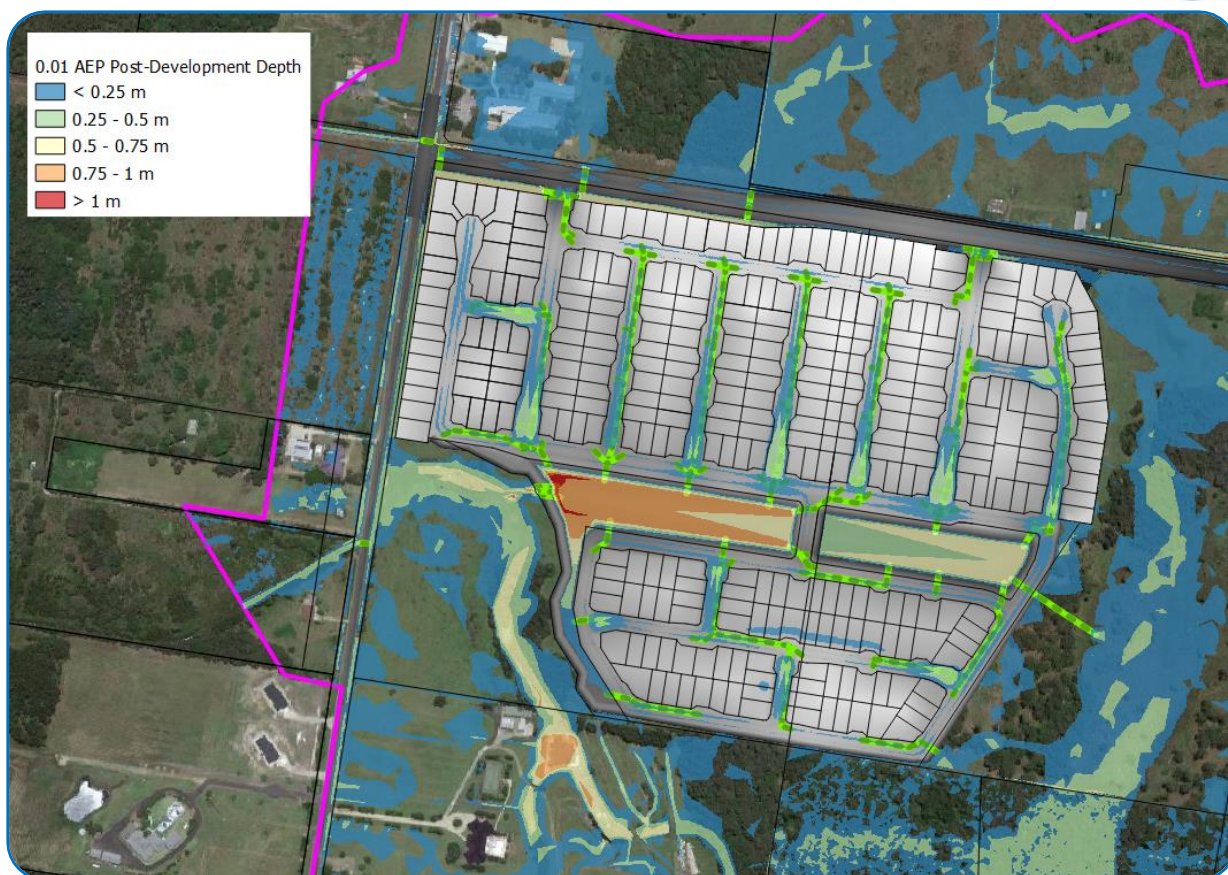
Figure 6.10 0.01 AEP Post-Development Peak Flood Depth
