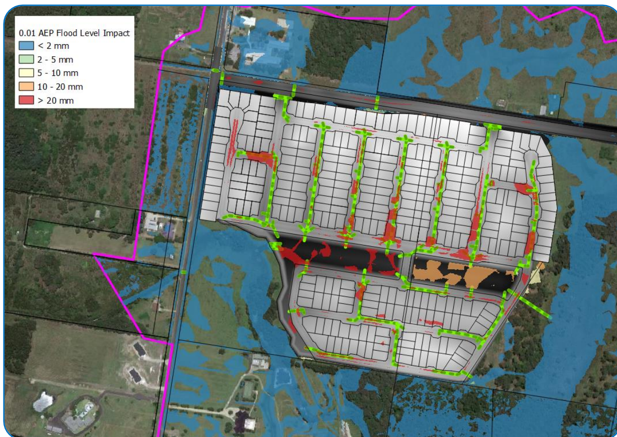
Figure 6.12 1% AEP Flood Level Afflux Plot
